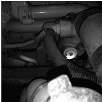
Figure 4: Location of coolant return plug
