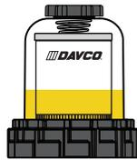
**Fuel level increases in clear cover.** As contaminants collect on the filter, the fuel rises to a non-contaminated section of the filter, providing optimal filtration while maintaining lowest restriction.
