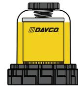
**The filter element is now completely covered by fuel.** At this point, all of the media's surface area is utilized. Restriction is increasing and the filter element should be changed at the next scheduled maintenance interval.
