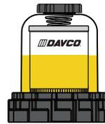
**Fuel level at filter wrap level.** Even though the fuel level is now more than half of the filter element, the fuel is still flowing through clean media at minimal restriction levels. The filter still has significant life remaining.
