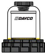
**When new, the fuel level in the filter will be very low with minimal restriction.** As the filter is used, contaminants collect on the filter from the bottom up. Fuel rises on the filter indicating remaining filter life.
