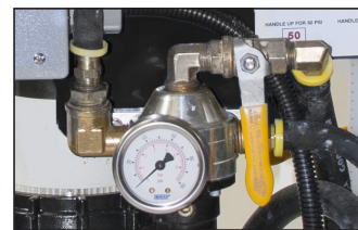
Optional 95/50 psi regulator for other engines
