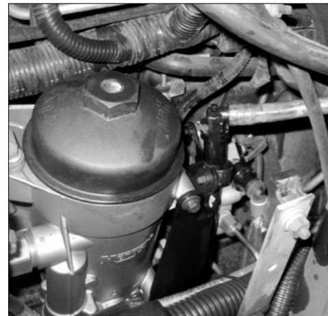
Figure 12: Re-route Return Fuel Line
