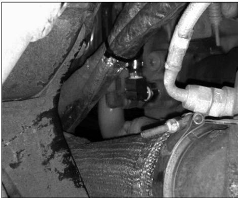
Figure 24: Secure the heater hose
